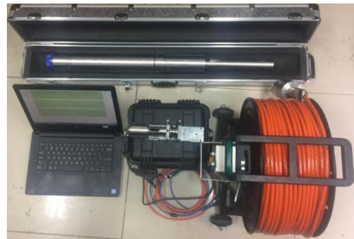
图 5 基于超声波 SAFT 钻孔成像系统实物图 Fig.5 Drilling imaging system based on ultrasonic SAFT
